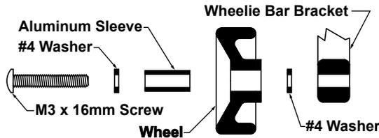
of the two wheelie bar brackets. Now install the screw assembly through the wheels and into the wheelie bar bracket in exactly the following order - M3 x 16mm buttonhead screw/ #4 washer/ aluminum sleeve/ **RPM** Wheel/ #4 washer/ **RPM** Wheelie Bar Bracket/ 3mm locknut. **Caution: The smooth, flat side of the #4 washers should face**
