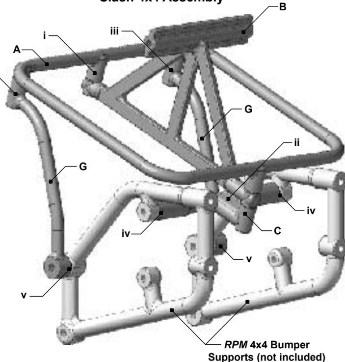
Letters  (A) Support Loop, (B) Tire Mount, (C) 4x4 Rear Brace, (D) 2wd Rear Brace, (E) 2wd Shock Tower Adapter, (F) 2wd Front Braces & (G) 4x4 Front Braces.
