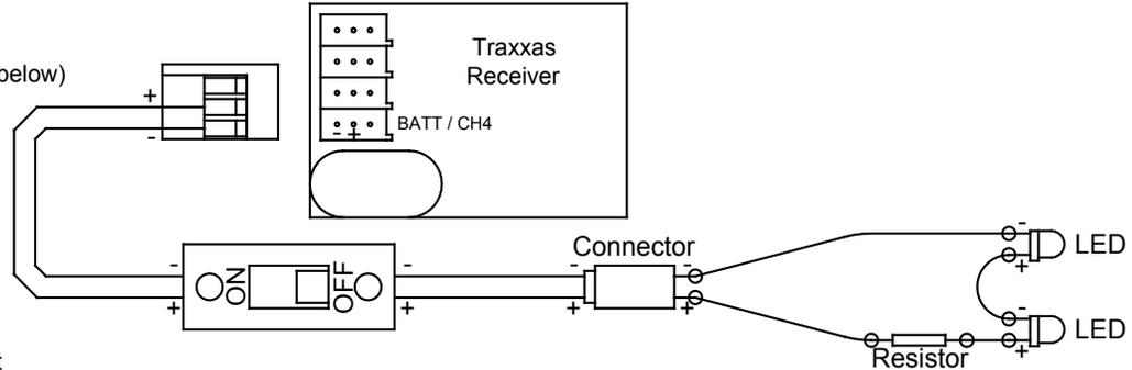
9) Solder your negative wire to the negative wire of the connector and solder the opposite end to the negative (cathode) of one of your LED's.
